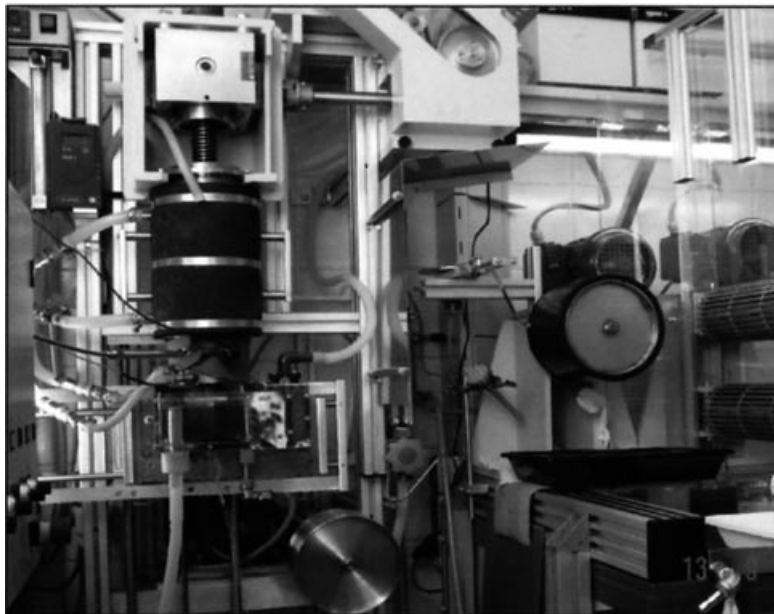
Figure 10. Laboratory spinning setup for the preparation of cellulose fibres and –filaments.
